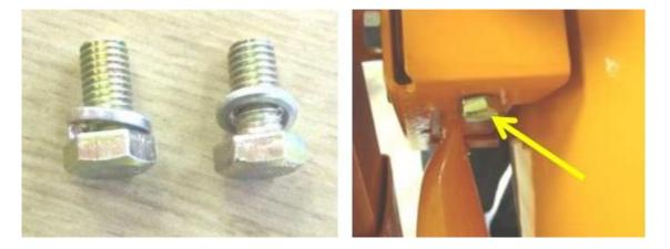
**Step-13** Place end cover(32) on the spring leg side to fix the drum(31) on other hand with 1 set of M8X70mm HEX bolts and M8.0mm nuts with Washer diameter 8.0mm.
