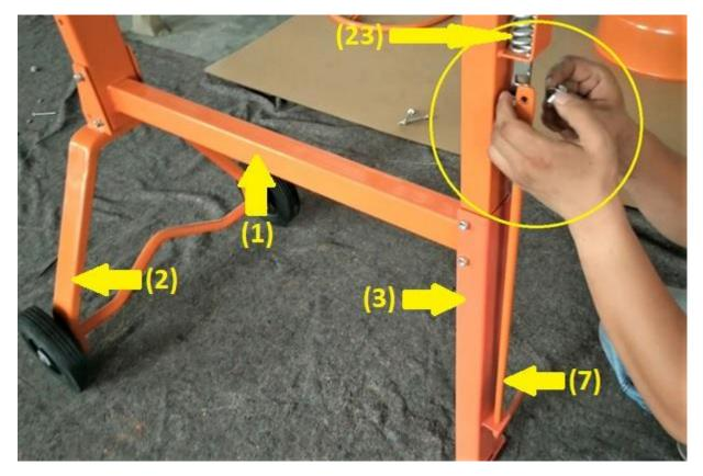
**<u>Step-8</u>** Place Electric motor panel(33 to 39 & 42) on the wheeled leg(2) side of the frame.
