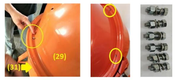
**Step-16** After assembling drum, attach the two mixing blades(30) inside the drum using 4 sets of M8x25mm oval bolts and M8.0mm nuts with washer diameter 8.0mm as shown in images below.
