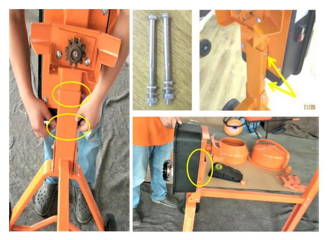
**<u>Step-10</u>** Attach the black cover(40) of the electric motor panel with the provided 0.75 inches long square drive pan head 7 screws.
