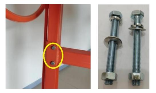
**<u>Step-5</u>** Assemble leg(2) with wheels(4) to upper frame part(1) as following picture.
