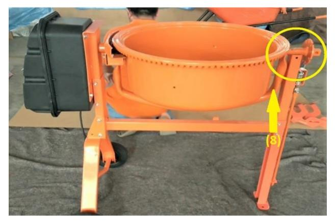
**<u>Step-12</u>** Fix the bottom of the drum(31) on both the gear side(9) by 2 sets of M8x25mm HEX bolts and washer diameter 8.0mm provided as shown in picture.
